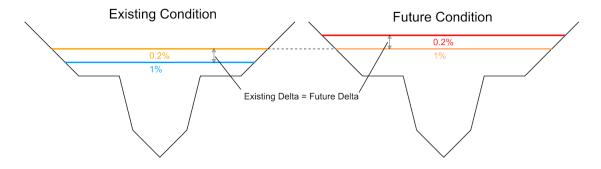
This process provides a more representative estimate of the future condition 0.2 percent ACE flood hazard area than a horizontal buffer, as it considers the elevation of the topography relative to the water surface. Where BLE data could be obtained, this process was implemented. These areas are listed below from south to north and are shown in *Figure 2.18*.
